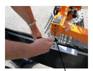
Remove the rubber guard cottar pin.
