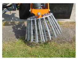
There are several different brush head settings, which determine different directions of spread.
