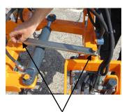
Remove the 2 ring pins on the steering rod. Remove the steering rod.
